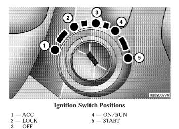
key to the right slightly, then remove the key as described. If a malfunction occurs, the system will trap the key in the ignition cylinder to warn you that this safety feature is inoperable. The engine can be started and 2 stopped, but the key cannot be removed until you obtain service.
